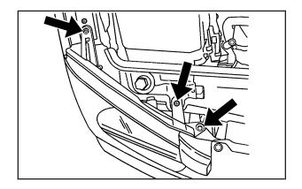
Remove the three headlamp assembly attachment screws. Pull the radiator cover/front grill toward you and pull the headlamp assembly up and out from the vehicle.
